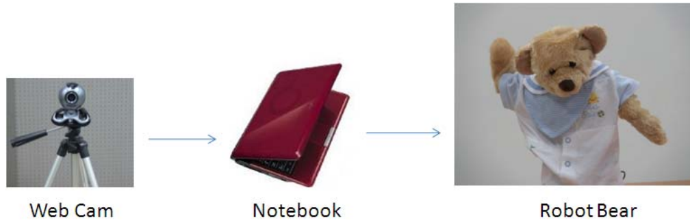
Fig.1. The RobotTell System which is composed of a Web camera, robotic bear, and a notebook.
