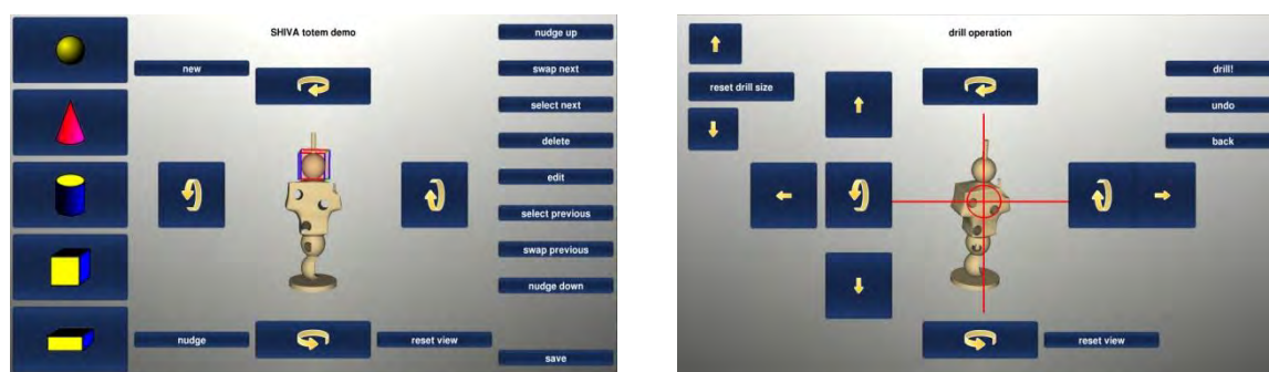
Figure 2. The totem-pole prototype interface. Left: main construction screen with buttons to add primitive geometric shapes to the stack, navigation buttons and a designed shape showing primitive stacking, blending and drilling. Right: drill operation screen with cross-hair controls for drill location and controls to rotate the object.
