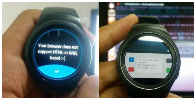
Figure 3. Samsung Gear S2 response when testing if native browser has XMLHttpRequest support using standard testing code provided in Tizen developers’ website (left). “Estimate It!” running on Samsung Gear S2 using Open-Source Webkit browser (right)
