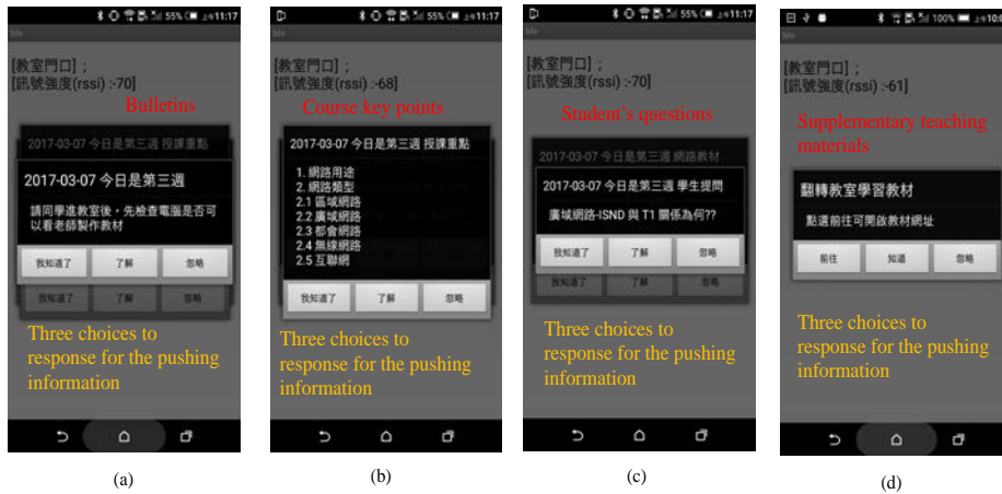
Figure 10. Student's APPs display three kinds of responses for four sorts of pushing information. (a) - (d) are four operating screens for four sorts of pushing information, bulletins, course key points, students' questions, and supplementary teaching materials, respectively.
