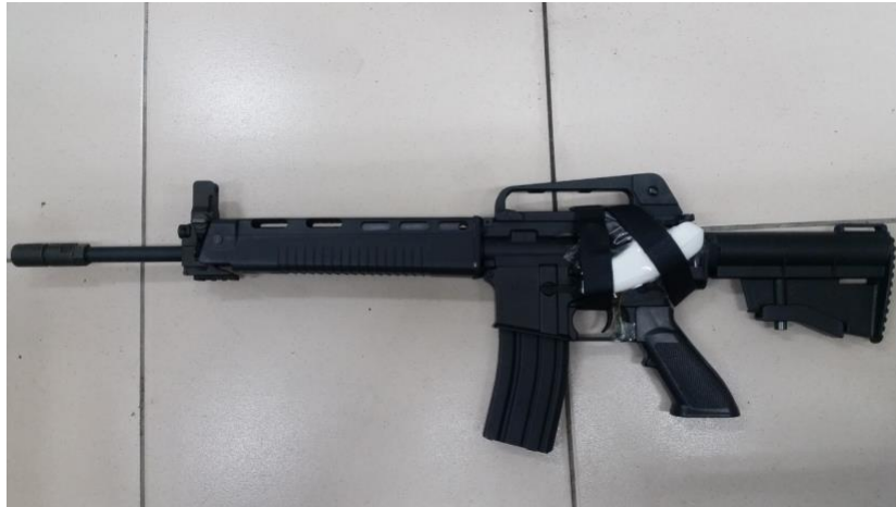
Figure 5. 1:1 real-scale T91 teaching rifles with Bluetooth function
