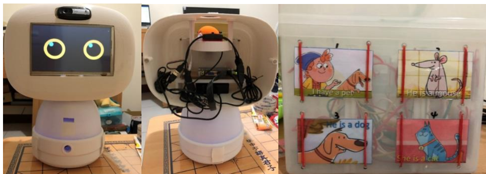
Figure 3. The design of the language learning robot and IoT toy.
